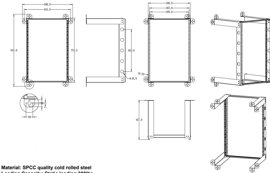
Loading Capacity: Static loading 300lbs
